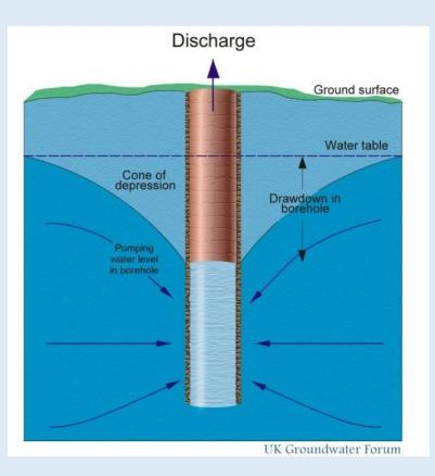
The pump lowers the water level in the borehole (initially, the water just comes from storage in the borehole)
