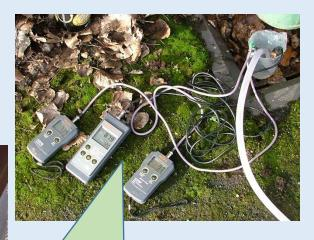
Some parameters must be measured on the spot (Temp, pH, EC, DO)
