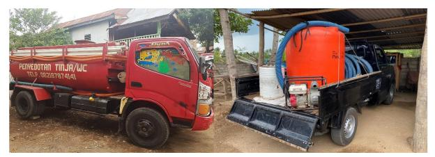
Pit emptying service providers use a 6-wheel truck with steel tank as in Makassar City (left picture), and use a pick-up with fiberglass tanks as in Lombok Timur Regency.
