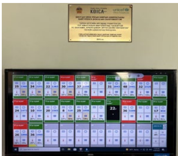
Figure 5: Real-time monitoring dashboard for smart water kiosk
