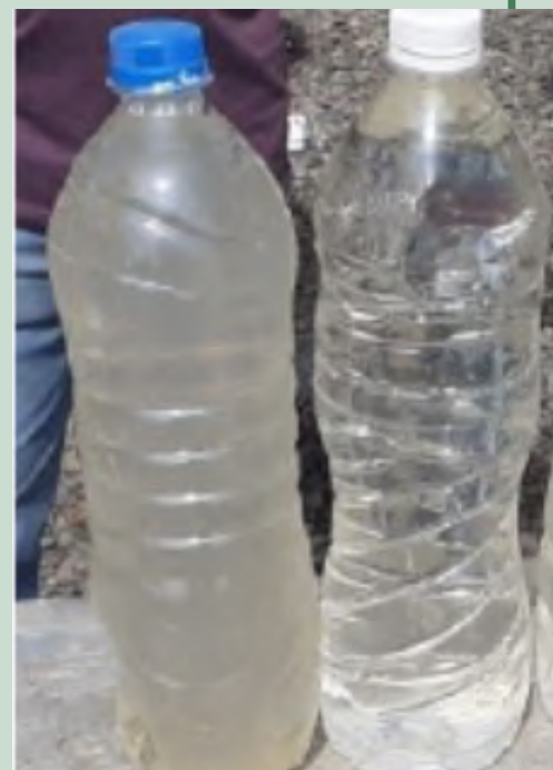
L-R:raw sewage sample; treated water sample
