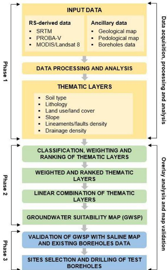
**Fig.5: Methodology of UNICEF Madagascar Remote Sensing Project**
