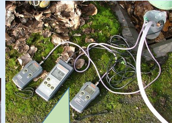
Some parameters must be measured on the spot (Temp, pH, EC, DO)
