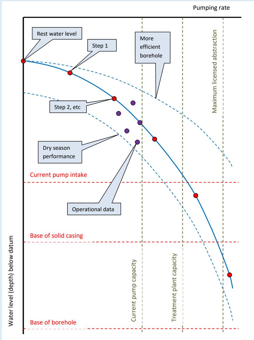
Another method of displaying test-pumping data:
